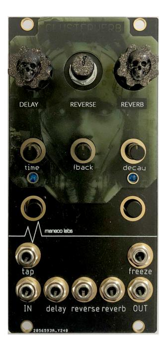
An effects processor with three simultaneous sections, reverse , delay with tap tempo and reverb with freeze , capable of the most complex sound landscapes but intuitive and user friendly at the same time.
